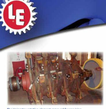
The Unigrator rotating element removed for servicing
