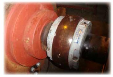
The factory was regreasing the Unigrator bearings at least three times per day prior to switching to LE's Almagard 3751 grease.
